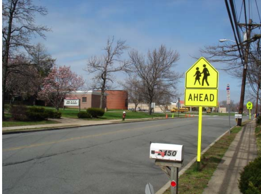
Photo 3 Example of School Advance Warning Assembly (Source: FHWA Safety Office)
