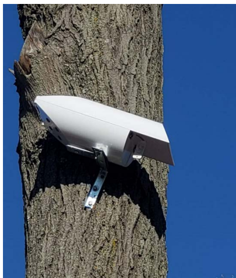
RWIS monitors provide the DPW with information on pavement conditions that helps make winter roadway treatment more efficient.
