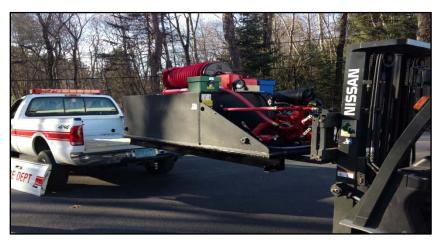
In early December, we took delivery of a new skid tank that slides into the back of a pickup truck to be used for fighting brush fires. The unit includes a 250 gallon water tank, a 200 gallon per minute water pump, and a 20 horsepower gasoline engine. This unit replaced one that was aging and unreliable. This skid tank is similar to other specialized fire equipment, we may not need it often, but when we need it there is nothing else
