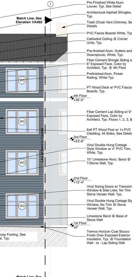
Trash Chute Vent Chimney, See - PVC Fascia Boards White, Typ. \_ Cathedral Ceiling @ Corner Pre-finished Alum. Gutters and Downspouts, White, Typ. Fiber Cement Shingle Siding w/ - 6" Exposed Face, Color by Architect, Typ. @ 4th Floor Prefinished Alum. Picket Railing, White Typ. PT Wood Deck w/ PVC Fascia Fiber Cement Lap Siding w/ 6" — Exposed Face, Color by Architect, Typ. Floors 1, 2, 3, & 4 6x6 PT Wood Post w/ 1x PVC Cladding, All Sides, See Detail
