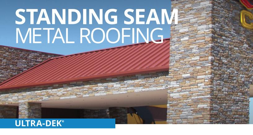
The Ultra-Dek® roof panel is a snap-together, trapezoidal leg standing seam roof system. Ultra-Dek® panels are available in 18-inch and 24-inch widths. Ultra-Dek® requires a minimum slope of ½:12 and is ideal for industrial, commercial and architectural applications. Ultra-Dek® can be erected on various types of construction.
