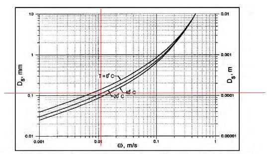
Figure 6.8. Fall velocity of sand-sized particles with specific gravity of 2.65 in metric units. Convert fall velocity from metric to US: 0.012 m/s = 0.039 ft/s
