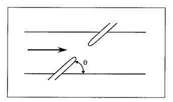
Figure 7.5. Orientation of embankment angle,  $\theta$ , to the flow.
