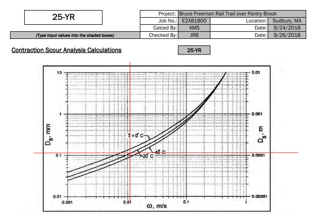
Figure 6.8. Fall velocity of sand-sized particles with specific gravity of 2.65 in metric units. Convert fall velocity from metric to US: 0.012 m/s = 0.039 ft/s
