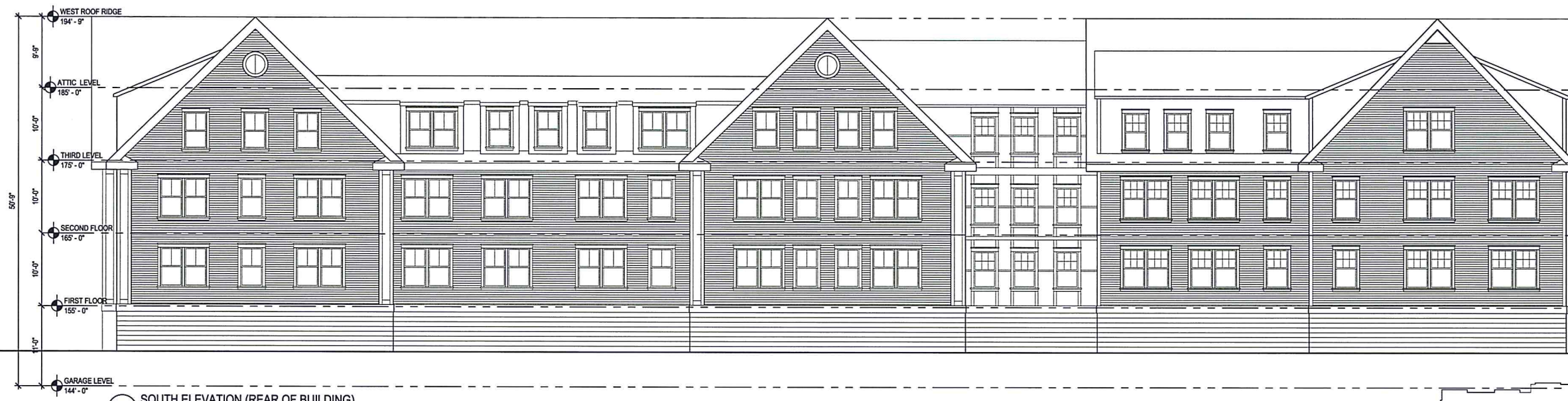
40 SOUTH ELEVATION (REAR OF BUILDING) SCALE: 1/8" = 1'-0"
