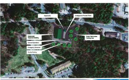
SUDBURY DECENTRALIZED WASTEWATER TREATMENT FACILITY -- CONCEPTUAL SITE PLAN WISTOR'SSMIPS
