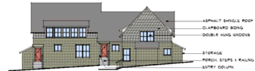
East Elevation-Bldg B Scale 3/32" = 1'-0"
