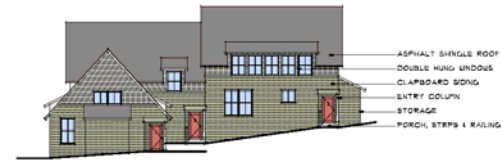
East Elevation-Bldg A Scale 3/32" = 1'-0"
