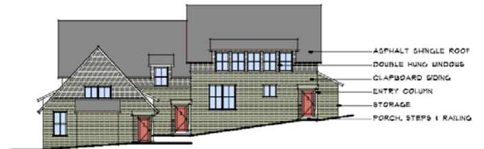
East Elevation-Bldg A Scale: 3/32" = 1'-0"
