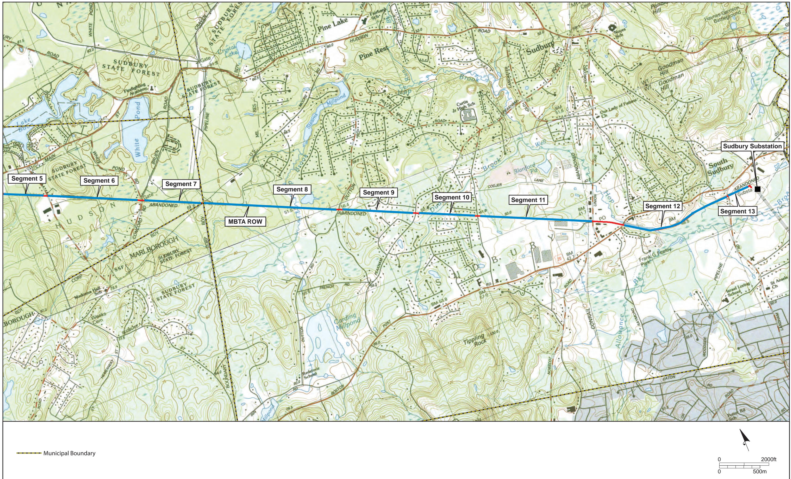
Figure 2. Proposed route of the Sudbury-Hudson Transmission Reliability Project in Sudbury, Marlborough, and Hudson on current USGS Quadrangle.
