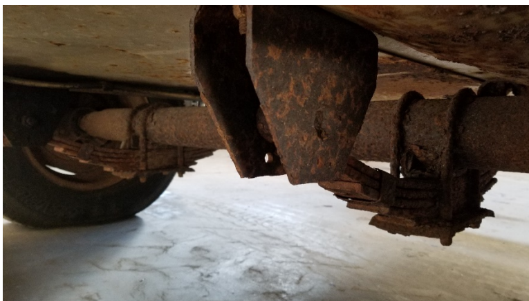
Rusted axle, leaf springs and mounts
