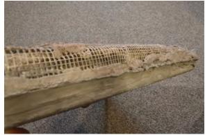
Photo 12 - EIFS base coat does not wrap around the board edges at the base of the system
