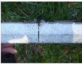
Photo 14 - Insulation Boards are spaced approximately 1/8 in.
