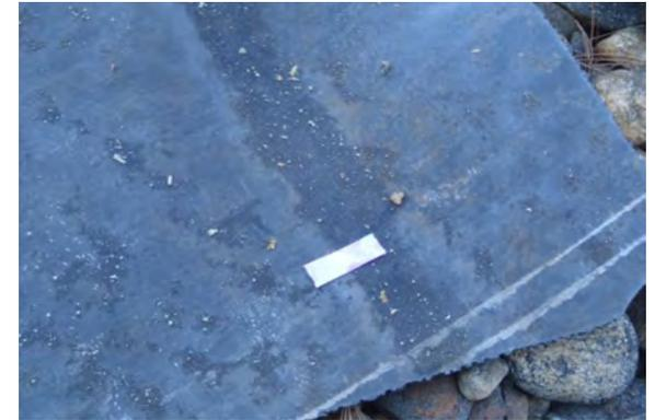
Photo 26 - Water test paper indicating condensation (pink color) on the underside of the EPDM membrane
