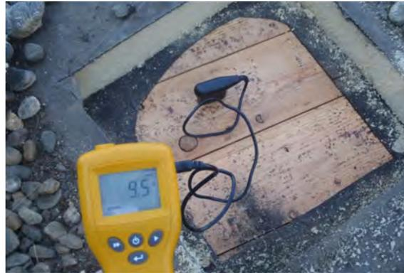
Photo 25 - Wood plank deck exposed at opening
