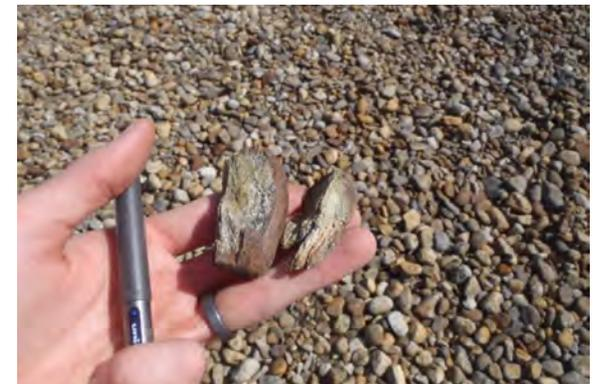
Photo 28 - Degraded roof ballast with sharp edges
