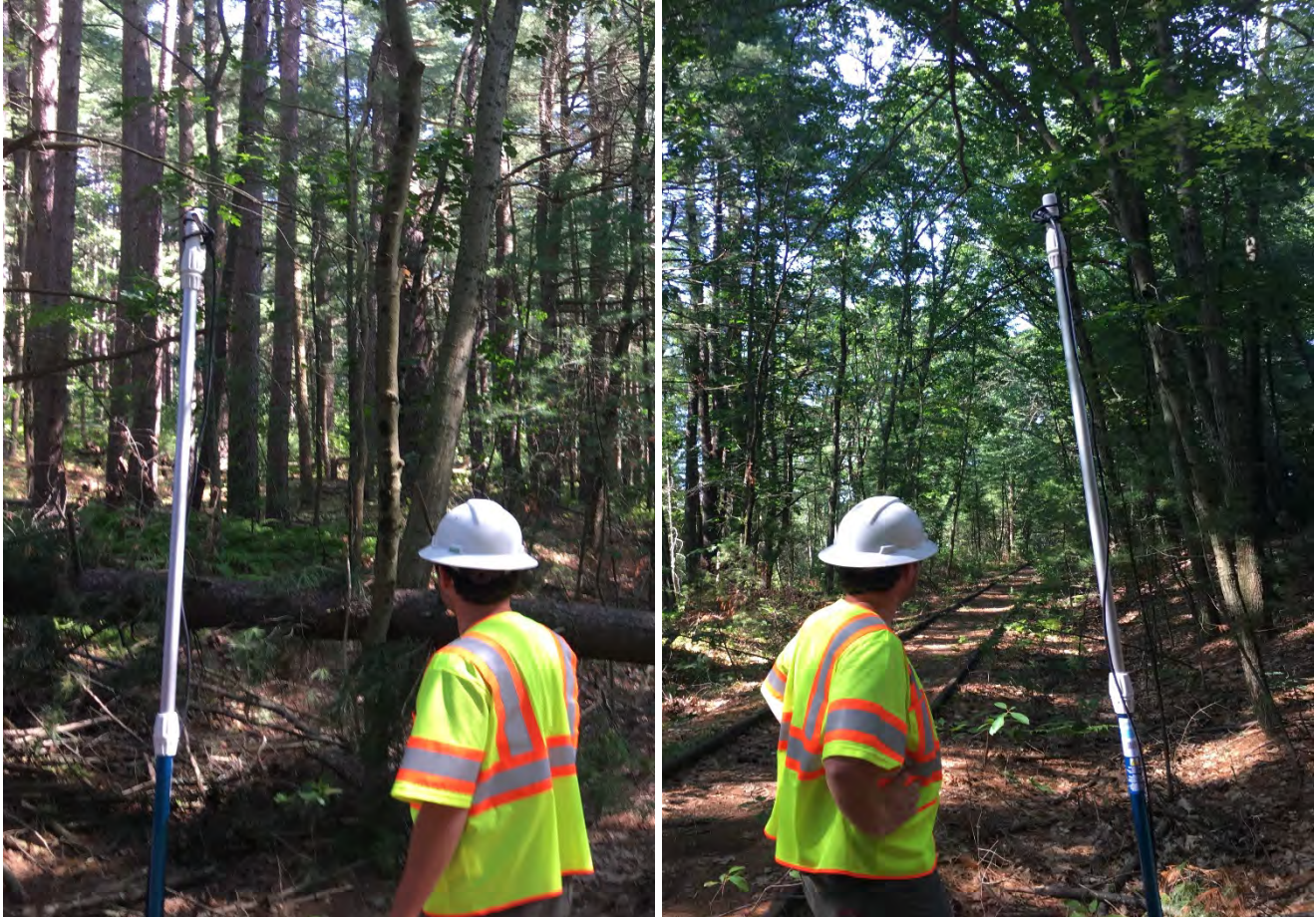
Site SU4: View of microphone (left) and detector view (right). The microphone is located at the top of the metal pole, approximately 3 m above vegetation height, angled horizontally to the ground and oriented towards the open railroad corridor to the north.
