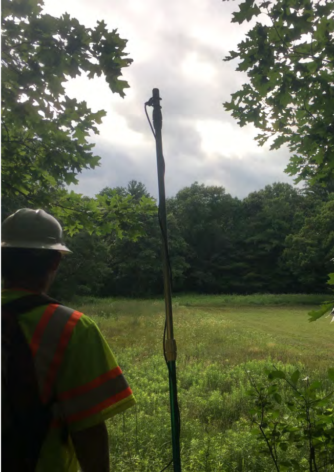
Site SU7: Detector view of site. The microphone is located at the top of the metal pole, approximately 3 m above vegetation height, angled horizontally to the ground and oriented towards the open playing field to the north. Note: No microphone view of detector obtained at this site.
