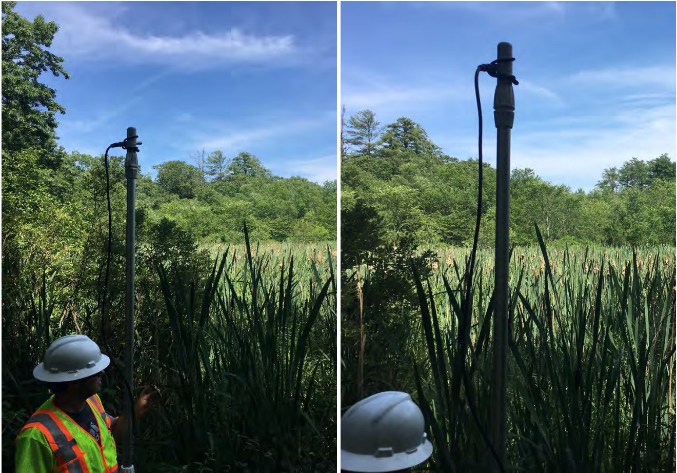
Site SU3: View of microphone (left) and detector view (right). The microphone is located at the top of the metal pole, approximately 3 m above vegetation height, angled horizontally to the ground and oriented towards a large wetland to the east.
