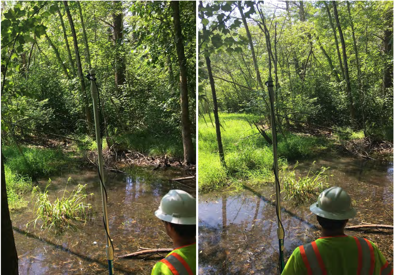
Site SU2: View of microphone (left) and detector view (right). The microphone is located at the top of the metal pole, approximately 3 m above vegetation height, angled horizontally to the ground and oriented towards a wetland to the east.
