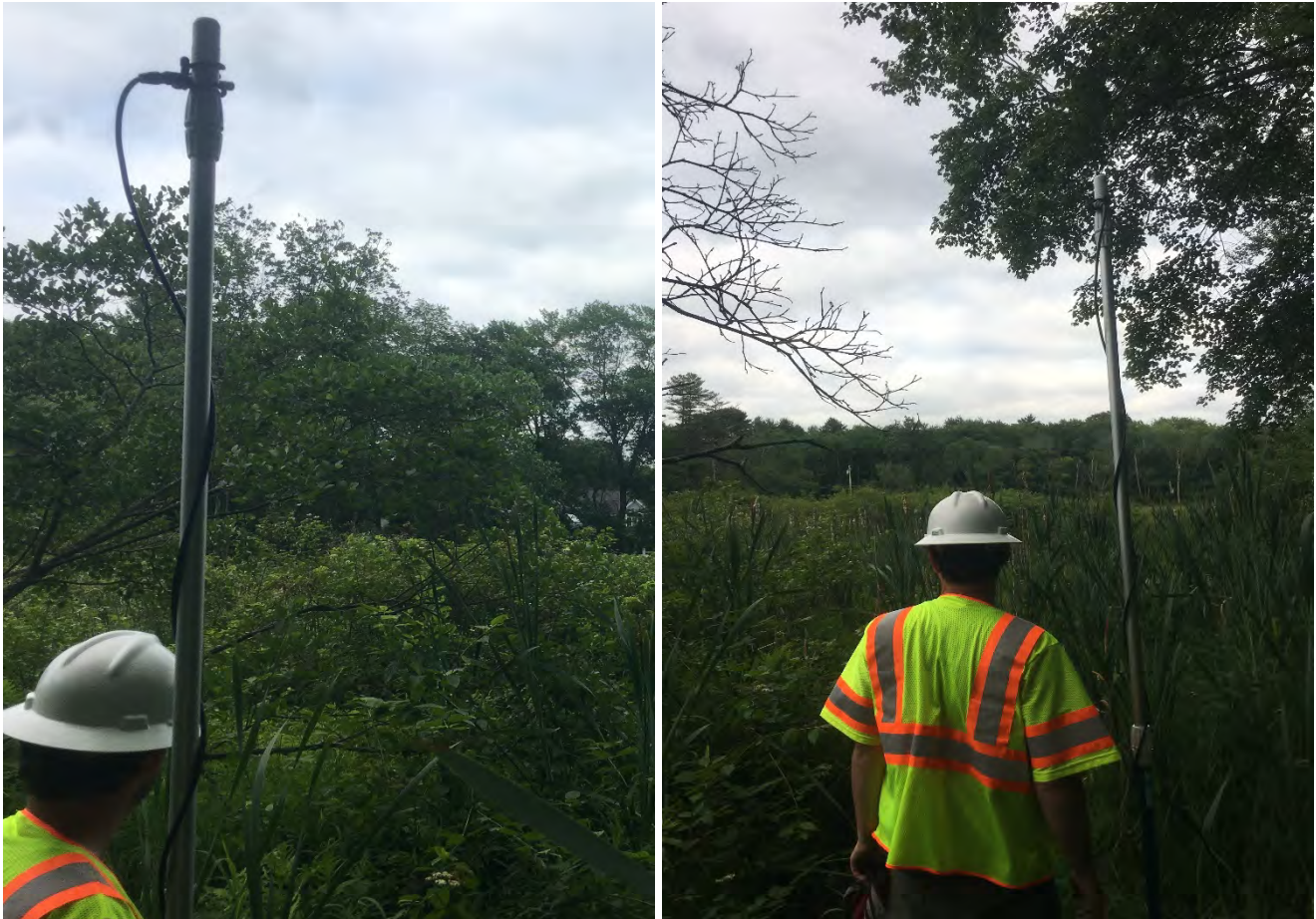
Site SU8: View of microphone (left) and detector view (right). The microphone is located at the top of the metal pole, approximately 3 m above vegetation height, angled horizontally to the ground and oriented towards the creek and riparian system to the east.
