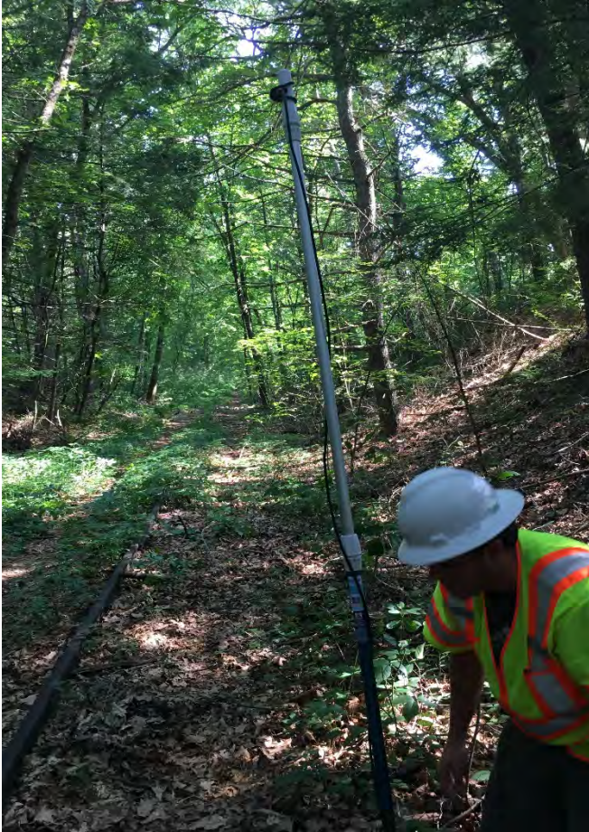
Site SU5: Detector view of site. The microphone is located at the top of the metal pole, approximately 3 m above vegetation height, angled horizontally to the ground and oriented towards the open railroad corridor to the south. Note: No microphone view of detector obtained at this site.
