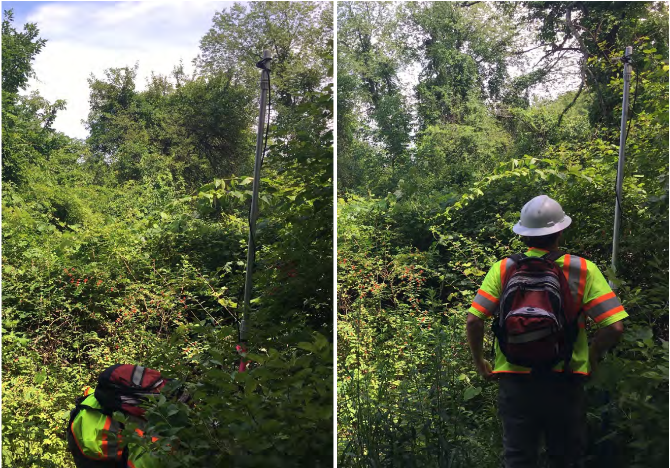
Site SU1: View of microphone (left) and detector view (right). The microphone is located at the top of the metal pole, approximately 3 m above vegetation height, angled horizontally to the ground and oriented towards the forest opening over a small creek to the east.
