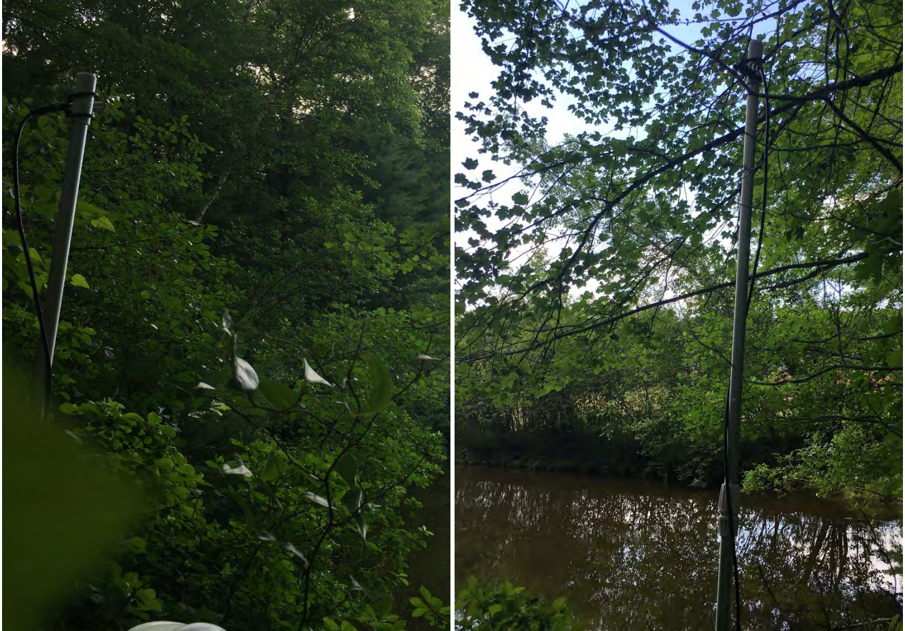
Site SU6: View of microphone (left) and detector view (right). The microphone is located at the top of the metal pole, approximately 3 m above vegetation height, angled horizontally to the ground and oriented towards the pond to the west.
