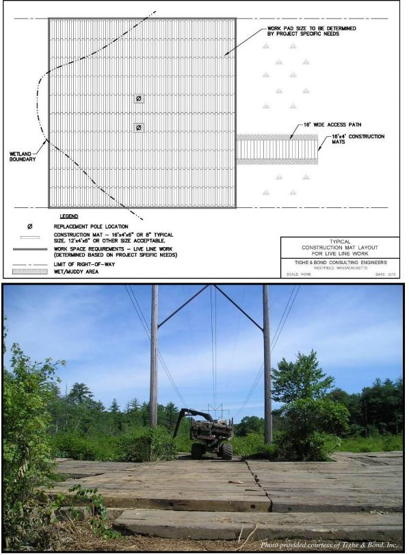
Construction mat wetland workpad for live line work.
