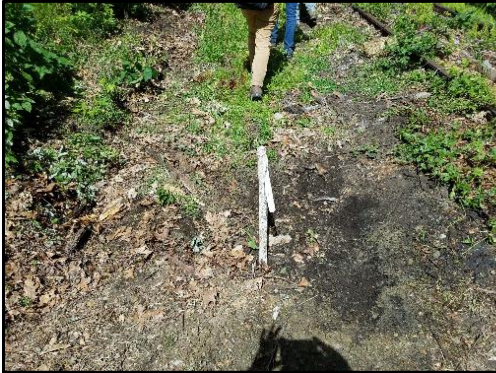
Representative photo of a boring in Hudson after it was advanced and backfilled
