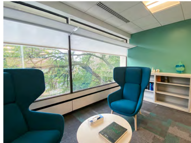
Harvard Office Renovation Interior light shelves reflect daylight deeper into the office floor plate. Team: FM, BVH
