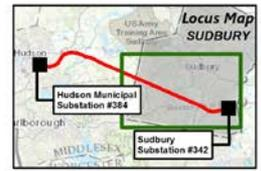
Proposed 115 kV Line Sudbury Substation #342 to Hudson Municipal Substation #384
